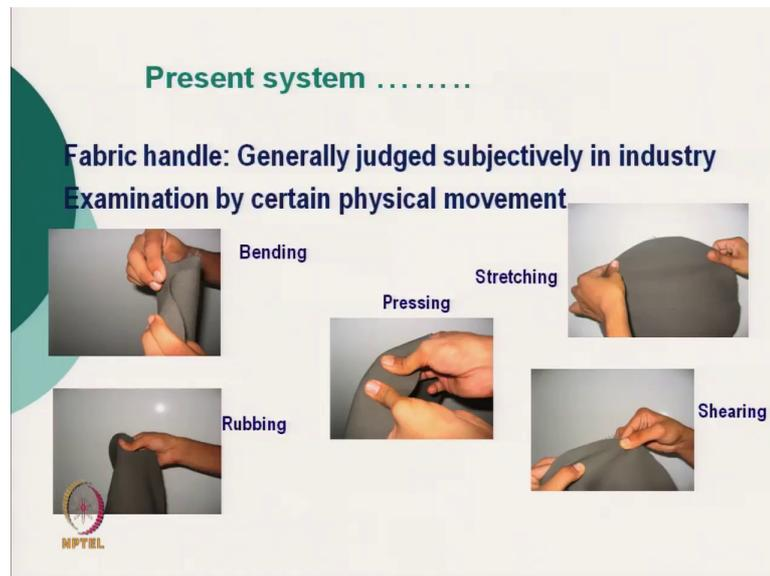
So, just I will this picture we will give the idea about the fabric handle characteristics when we select normally we select fabric based on all these characteristics by bending we try to bend the fabric by finger to see that whether it is a flexible or not, stretching we try to stretch the fabric, we try to press the fabric whether it is a compressible or not whether it is a soft or not.
