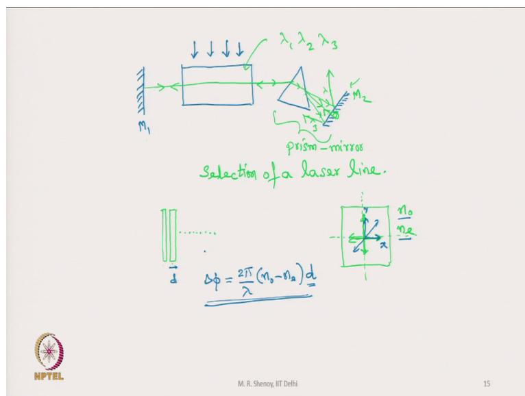
So, let this be the laser system here and this is mirror m 1; it is a very nice arrangement and so, there is a laser beam. At the other end we have a prism and then there is a mirror. This is
