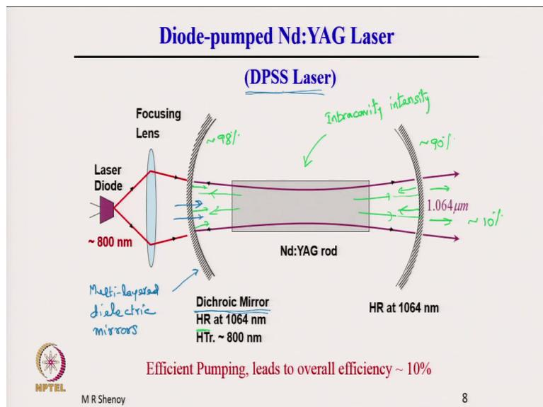
So, what is now shown is the diode pumped YAG laser. So, diode pumped solid state laser, this is in the class of diode pumped solid state laser. So, a schematic is represented here, again it is not correct to scale. So, we have a laser diode pumping around 800 nanometer and the laser light is focused here on to the Nd:YAG rod.
