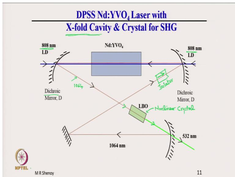
So, here what I have shown is an X fold cavity as you can see this is like an X; so, it is a folded cavity. The advantage of folded cavity is if we were to have more number of components along the same line, then the length of the system becomes much larger and it goes beyond the experimental table that we have. And therefore, if you have a folded cavity, then you can have much more compact setups.
