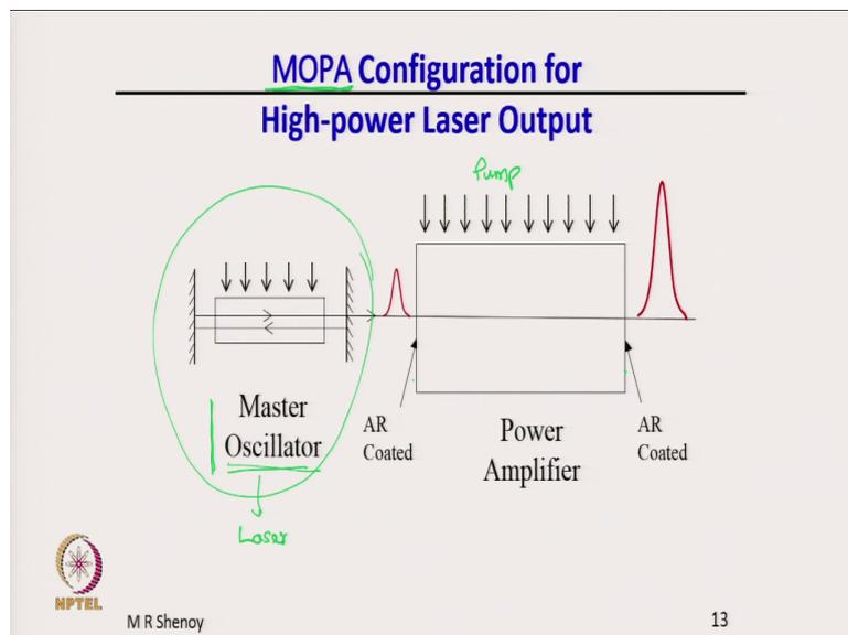
Here in this diagram, what I have shown is what is called as MOPA configuration. MOPA stands for Master Oscillator Power Amplifier configuration for high power laser output; so it is illustrated here. So, there is a master oscillator is a laser. So, here oscillator refers to the laser. So, when you need very high power laser output.
