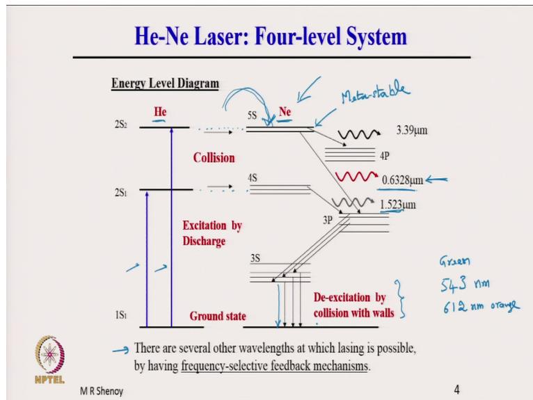
So, let me first take the He-Ne laser, helium neon laser. Almost all of us have seen this orange red coloured output from a helium neon laser. It is an example of a four level laser. Why He-Ne? Which is the active medium? The active medium is actually neon, the lines that we see. The laser lines that we get are transition lines corresponding to the excited neon head.
