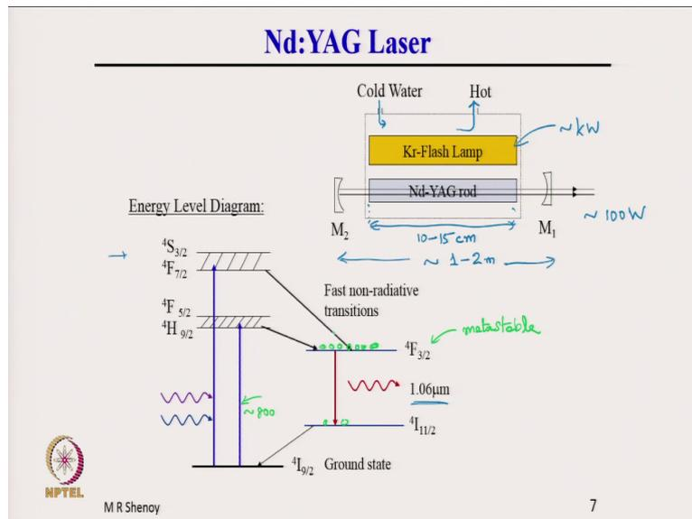
So, here I have shown a schematic of the Nd:YAG laser; this is a flash lamp pumped Nd:YAG laser where you have a Nd:YAG rod, this is not correct to dimensions. So, this rod length is typically 10 to 15 centimeters, the length of the rod and here is the flash lamp. The flash lamp pumped cavity is generally of the order of 1 to 2 meters in length; the cavity length is much longer compared to the rod.
