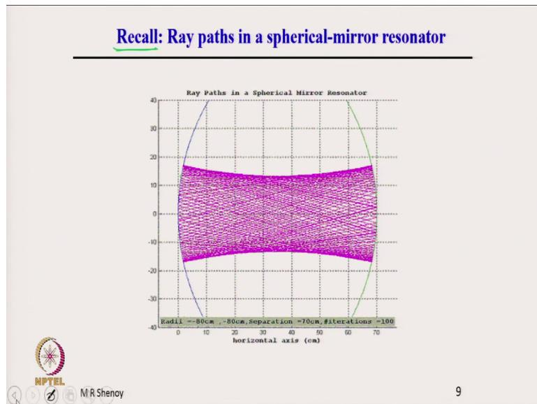
So, what is shown here is just to recall the ray paths which we had seen earlier in the spherical mirror resonator that the beam looks like a Gaussian beam which goes back and forth, when you draw the ray paths. And that is why we have shown here, a Gaussian beam which is going back and forth inside the spherical mirror resonator.
