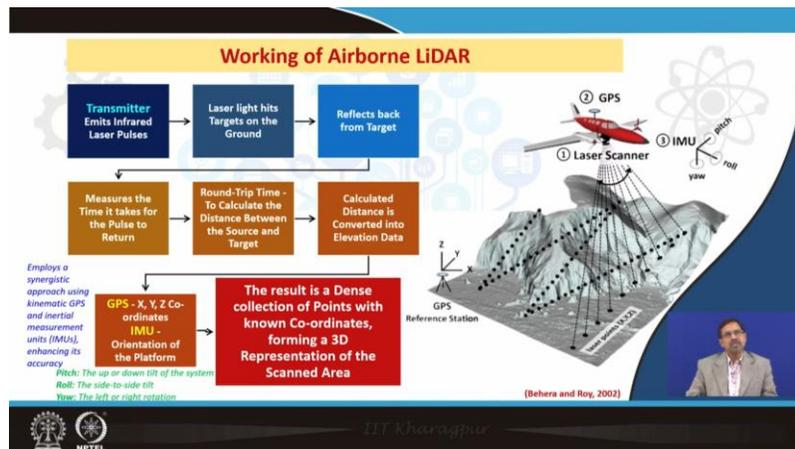
yaw is the left or right rotation. This actually happens in terms of the airborne LiDAR, where the tilt, the side-to-side roll, and yaw are sometimes also calculated in terms of
