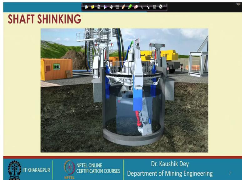
For cutting the set profile in the required section; the shaft is kept full of water during sinking to balance the level of the ground water table in the surrounding geology. In addition.
