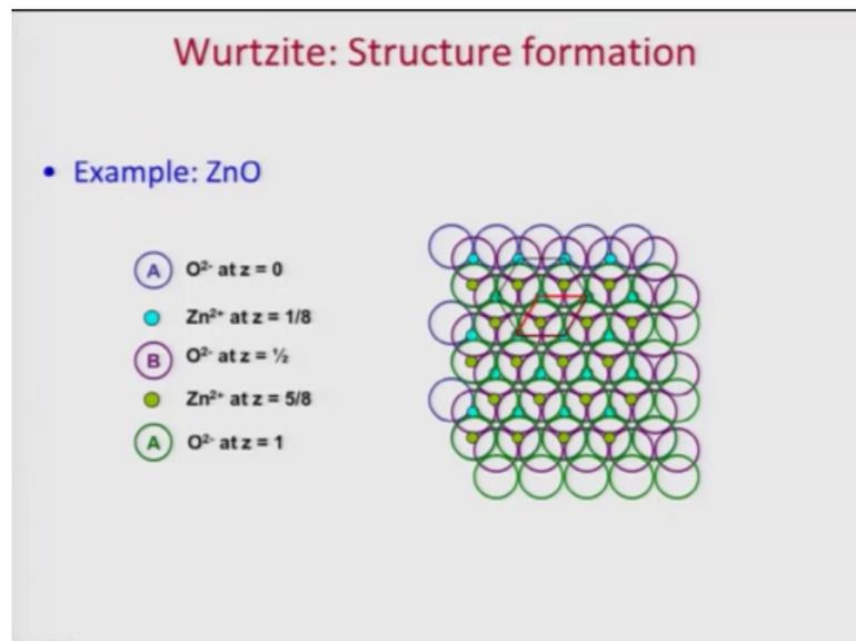
So, let us see how does it work in case of ZnO. So, first layer of oxygen goes at z is equal to 0. Second layer of zinc goes at z is equal to 1 by 8. Third layer of oxygen goes at z is equal to half and the next layer of zinc goes at 5 by 8 and then again oxygen at z is equal to 1. So, this is how you are going to have these unit cells.
