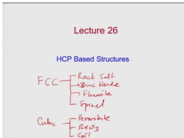
Starting, continuing the same things that we are talking about in the previous lectures about structure of ceramic materials. So, in this case we throw into; so today we are going to talk about materials which are at HCP Based Structures which are based on a HCP packing of anions. So, so far what we have discussed is basically the structures which are based on FCC packing of anions, so we looked at all the structure such as rock salt, zinc blend, and fluorite and finally spinel.
