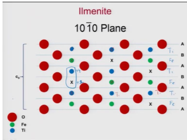
So, again if we draw the  $10\bar{1}0$  plane and just like in previous case you have first layer of aluminum oxygen. Next layer of iron all right. Next layer of oxygen, again next layer of what has happened here again this should be so; next layer of titan this is our titanium. So, I think the colors have one different, this is titanium, this is titanium and this would be empty in this case.
