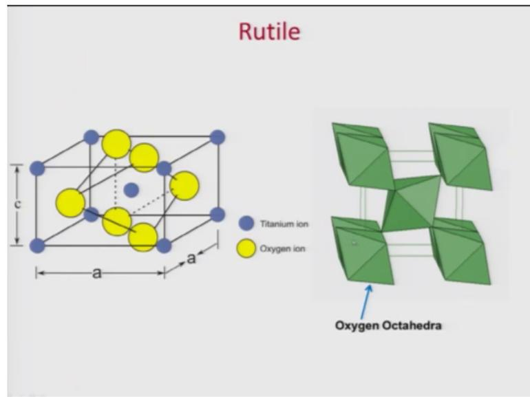
And this is how it looks like. So, you have a unit cell tetragonal unit cell which can be made by cations. And anions are located, two of these anions are located on these two faces, so you can see one is shifted by down there another is shifted up there. And the other two cations are on these two faces and they make sort of an octahedron and this is.
