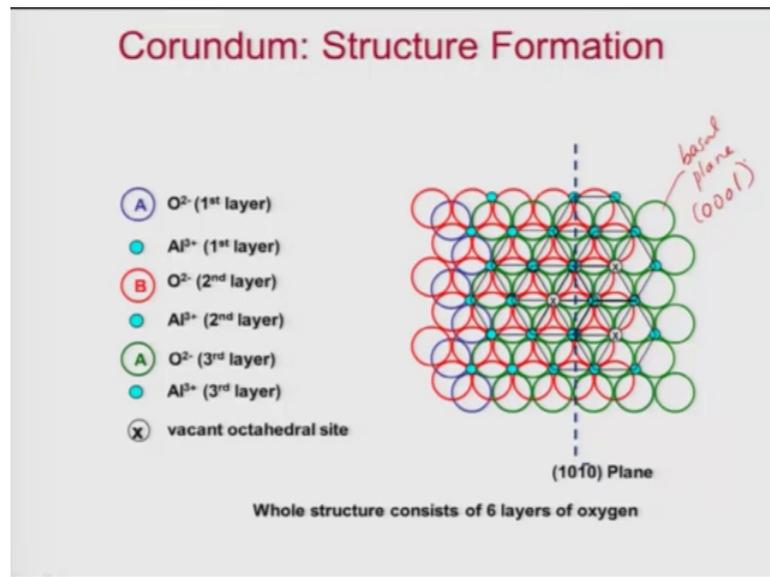
So, let us see how the structure is made in this case the oxygen layer is the first layer. So, this is the A layer of oxygen. And then you have aluminum going to the octahedral voids in the 1st layer. So, this is let say the octahedral void of the 1st layer.
