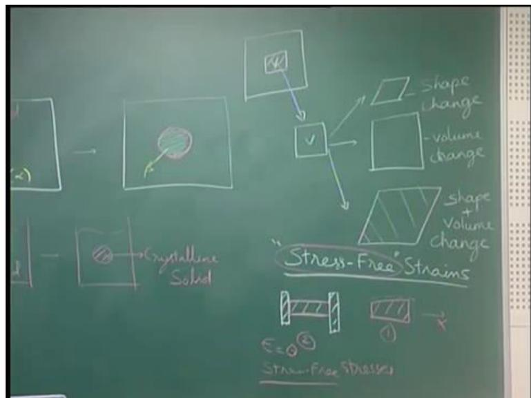
So, I have a volume  $v$  of material, which I have plugged out from the material from the inside of the matrix, I can have this volume  $v$  of material transforming just by pure shape change that means, I assume that the volume is constant I could have a pure volume increase that means, the shape is same or I could have a combination, where in I have a
