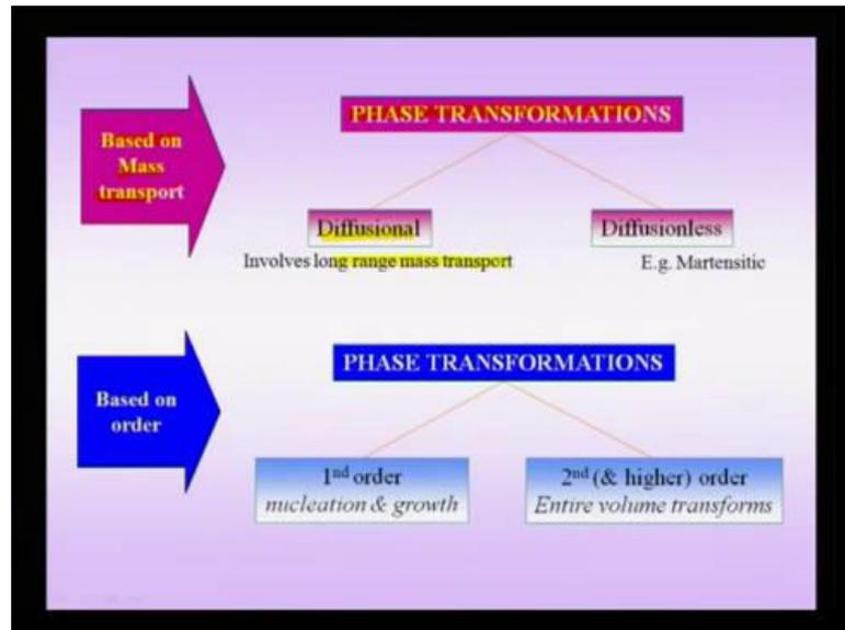
So, this slide brings out some of these in a pictorial form, that based on mass transport I can classify phase transformation as diffusional and when I mean diffusional, I am typically talking about long range mass transport or diffusional, diffusion less. For instance, we will consider in this chapter a particular kind of diffusion less transformation known as the Martensitic transformation, further thermodynamically based on order, we can classify phase transformations as first order.
