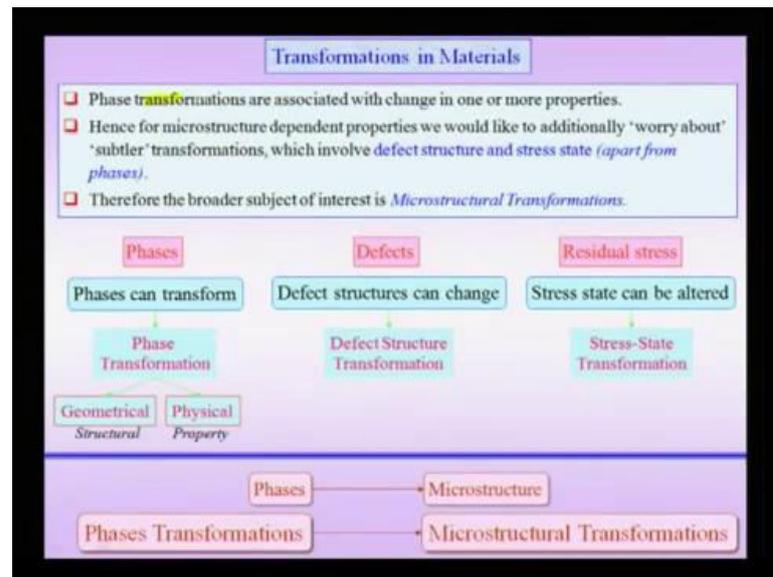
Phase transformations are associated with change in one or more properties of a this is the reason, that we are studying phase transformation that we want to engineer the properties. And if therefore, microstructure dependant properties, we would additionally like to think about and we would also worry, how as to how the defect structure and the stress state change apart from the phases, in other words I need not only worry about the phase transformation.
