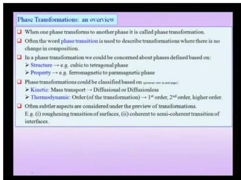
So, let us start with a overview of phase transformations, when one phase transforms to the other we call it an phase transformation, often the phase transformation is used to describe transformations, where in there is no change in composition. And we will take
