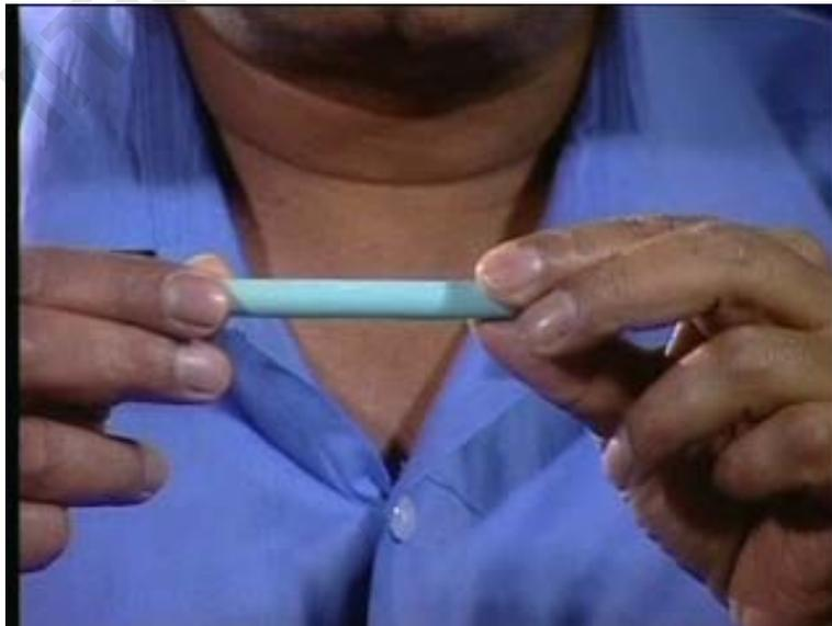
i have chosen a material chalk a simple chalk has been chosen and which apply a pio torsion onto the chalk
