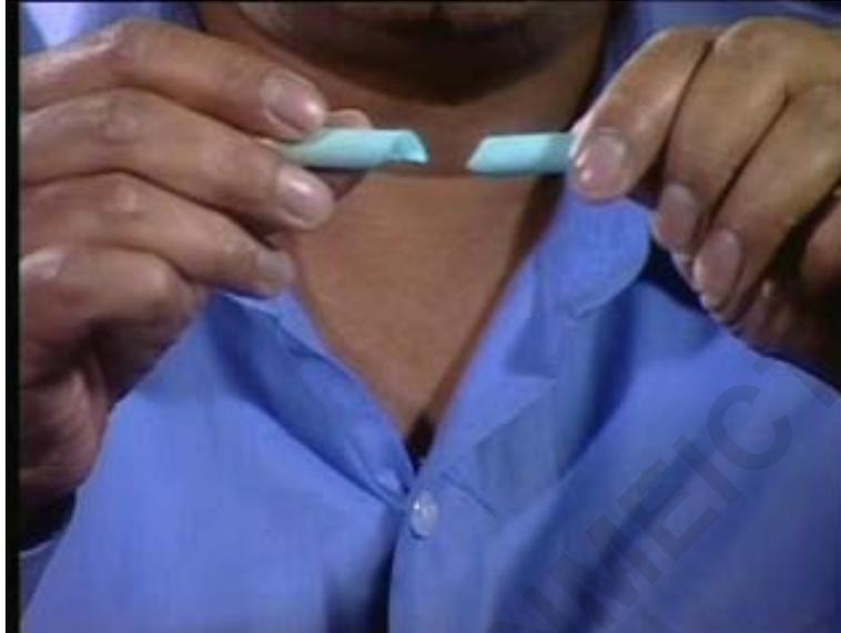
just you can see that if i apply pio torsion then it's little hard so just see it has broken can you see the broken portion how it as failed so it as just failed in the situation of this forty-five degree line i mean i mean this both way this is a forty-five degree line so what is happening if you consider this forty-five degree line can we not see it is resembling the same forty-five degree line what we have drawn on to this particular plate over here okay
