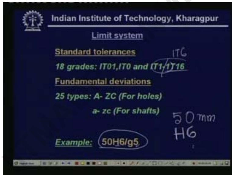
a limit system is defined by standard tolerances which are of the eighteen grades higher the grades means higher the tolerances and fundamental deviations are of the twenty-five types as i mentioned A to ZC
