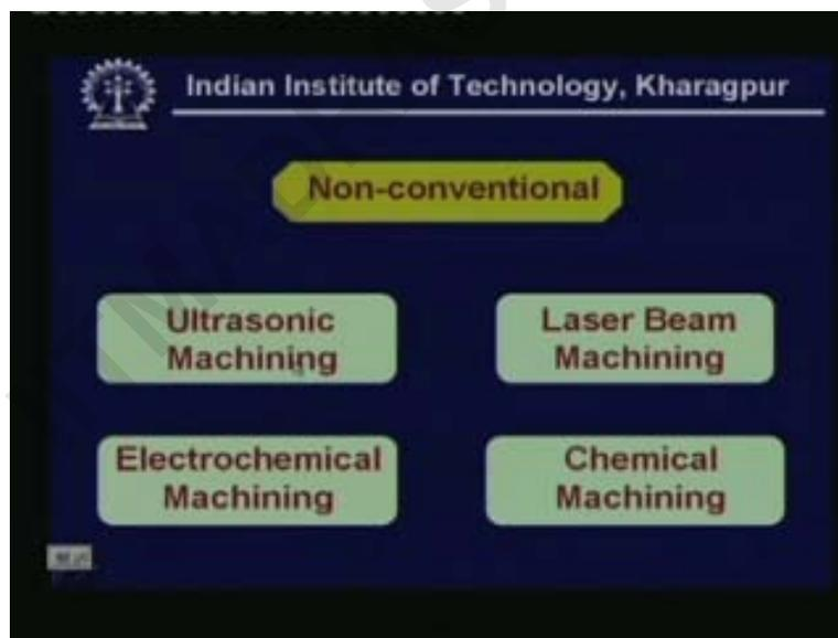
and lastly i go for a non-conventional procedures which you can see are given over here as ultrasonic machining laser beam machining electrochemical machining and chemical machining there are several other varieties you know the ultrasonic uh machining utilize an chemical energy the labor laser beam machining utilizes a thermal energy so this is an thermal energy this
