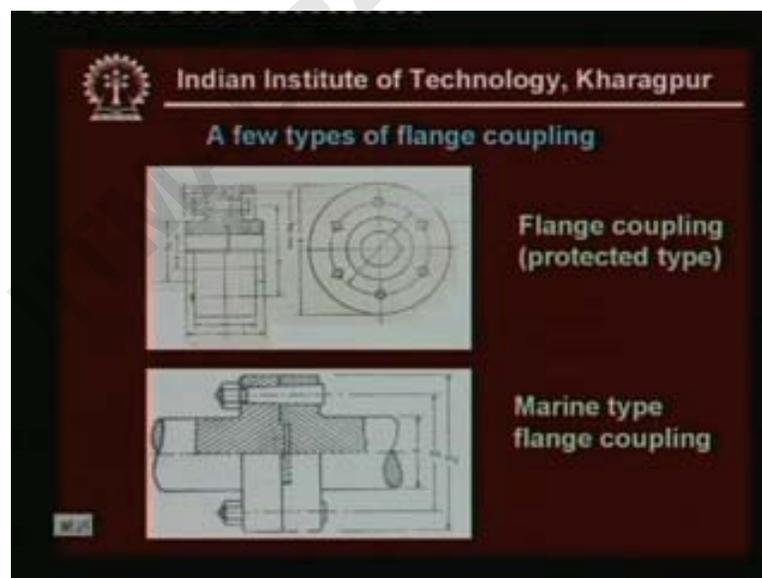
now let us come to few types of flange coupling now flange coupling you see ah these are the ah couplings again rigid couplings and the coupling is done by means of two flanges
