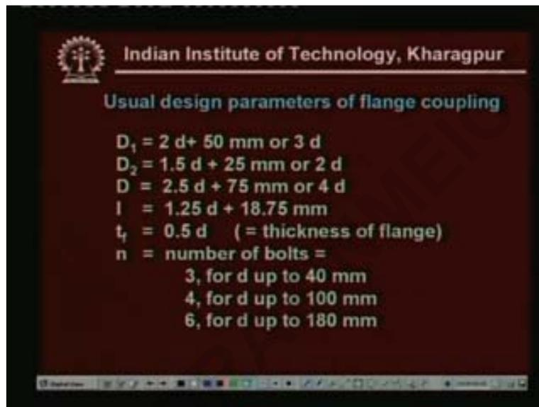
$D_1$  as I said which is equal to the bolt circle diameter this is roughly taken to be twice  $D_2$  small  $d$  that is the diameter of the shaft plus fifty in millimeter that is fifty millimeter or it may be three  $d$
