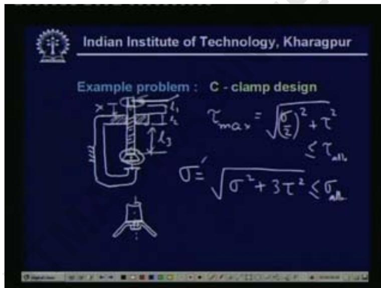
now there are few failure criteria's which you have say we have tau max this is the failure by maximum shear stress and this will be equal to sigma
