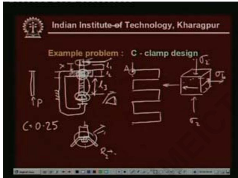
if you consider the cross section of the thread then this point will have the compressive stress suppose it is here then the compressive stress is {maxim} (00:29:47 min) P there will be compressive stress so if you have one element at point A if you draw the state of stress there will be compressive stress
