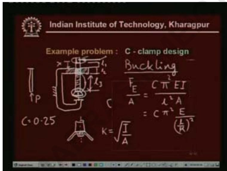
so the buckling is one of the important criteria which has to be considered here because this part is subjected to the compressive stress
