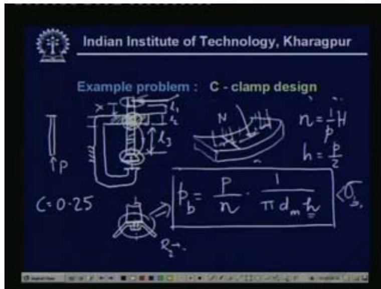
so if you consider a single thread then the total force on the single thread will be equal to  $P$  by  $n$  where  $n$  is the number of threads in engagement with the nut [noise] and it depends upon the pitch that is  $n$  will be equal to one upon pitch that is equal to number of thread per unit length and times the height of the nut that is this length
