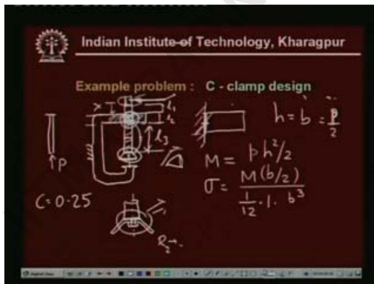
it is easy to calculate the bending stress first comes bending moment which is equal to  $P h^2$  by two therefore the bending stress is  $M$  and here the maximum bending stress will be at  $b$  by two divided by  $i$  which is equal to twelve times one times  $b^3$
