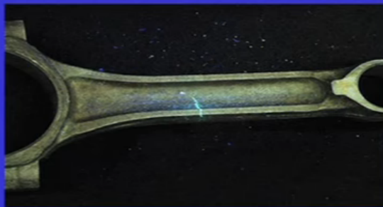
Fluorescent penetrant indication
