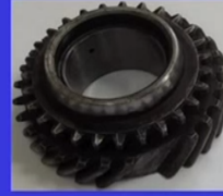
Two teeth broken in the 2 nd gear
