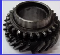
One tooth broken in the 2 nd gear
