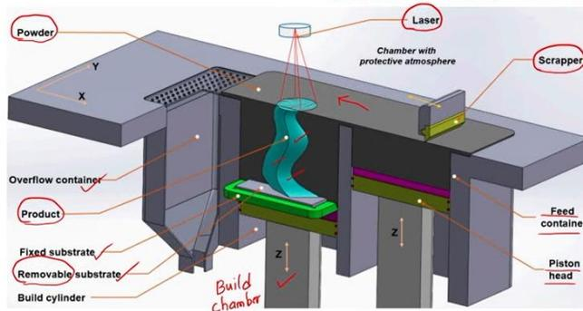
Figure. Schematic of Selective Laser Melting (SLM)
