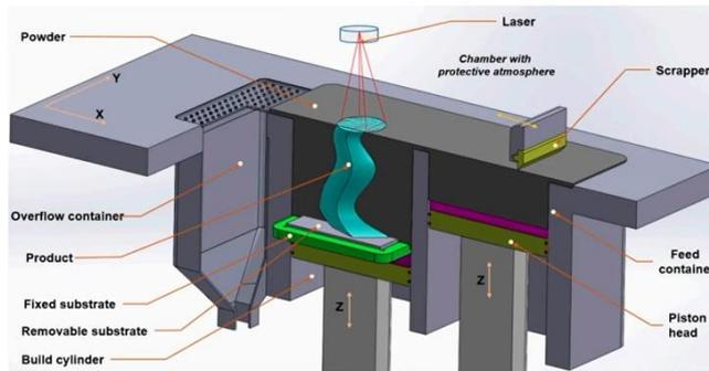
Figure. Schematic of Selective Laser Melting (SLM)
