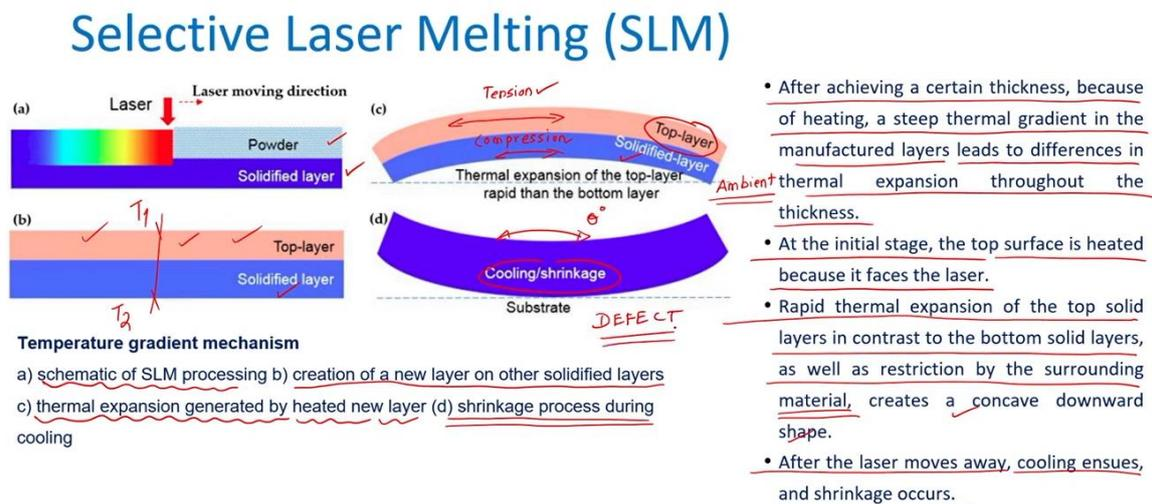
However, there is a little limitation of the SLM, when we want to develop the thin products or thin cross sections, there may be chances of distortion or deformation, uncontrollable deformation of the work parts, and it is primarily due to the TGM, that is a temperature gradient mechanism which we have seen in our laser based forming operation.
