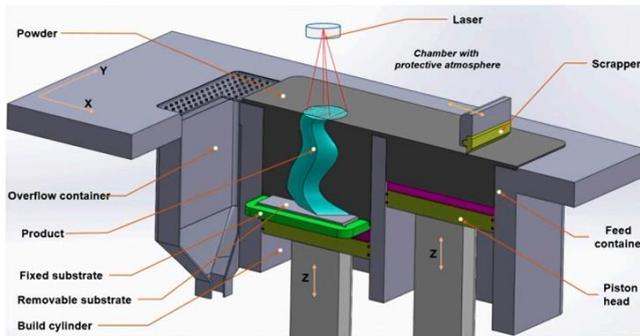
Figure. Schematic of Selective Laser Melting (SLM)
