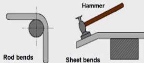
Then there are bending operation, normally which is done with the help of a hammer. If it is sheet bending, you bend it, or if it is a rod you can bend it on a roller and get the shape.
