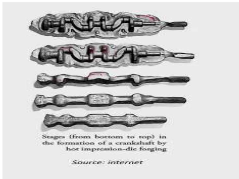
This is the typical case for the formation of a crankshaft, source is internet only. The initial operations are done okay, various operations like fullering, drawing, swaging and other things are done, drawing operations are done. So this part takes care of for this crankshaft portion and like this. So this is your blocking operation, this is your finishing die impression which you're getting, and then after that it will be trimmed off okay. So this is the final forging operation which comes.
