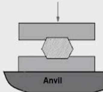
Then is the swaging. Swaging is done to reduce the finish work for desired size and shape, usually either round or hexagonal shape they obtain for that the swaging, may be to some extent there is the die cavity is there, so you get the very good shape for that. For small jobs, top and bottom swage pair is employed, whereas for large works swage block can be used.
