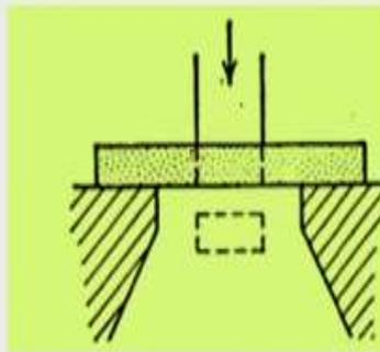
Then there are punching operation. The metal is kept on a die and this is the work piece material, it is kept on a die and punching tool no it moves downward and then causes shearing of the material resulting in a small die. Depending upon the shape of the punch, you will get a hole which is made there, so that is the punching operation which is done.
