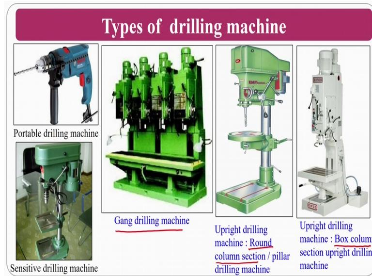
Types of drills if you see portable drilling machines is there, sensitive drilling machines are there, gang drilling is there; that means, that as just now I was telling about some gang. So, where you can have multiple operations can be done in a single go that is upright drilling with a round column is there, at the same time you have a rectangular box column also will be there these are the varieties of the drilling machines are available in the market.
