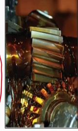
These are the varieties of things that will be used less accuracy and finish is there. The same time you can see here how the gear hobbing takes place? How the cutter is cutting in a single go.
