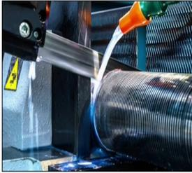
So, if you see the cutting fluids in the sawing process, the sawing process normally do not uses the cutting fluid whenever you are operating for the wood; however, whenever you want to chop it off from the very very big large size blanks to the small, small workpieces and all those things in the metallic region normally you should go for suitable cutting oils.
