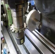
Cutting of gear by milling
