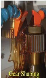
**1. Gear Shaping (Pinion Cutter):**
