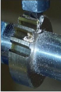
Cutting of gear by shaping
