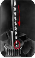
So, when the broaching process will be normally used in normally whenever you want very very big holes of different different shapes and all those things, where you cannot drill or you cannot do the other processes normally you can go for broaching operation. It moves a multiple tooth cutting tool linearly to workpiece, work in the direction of tool axis ok.
