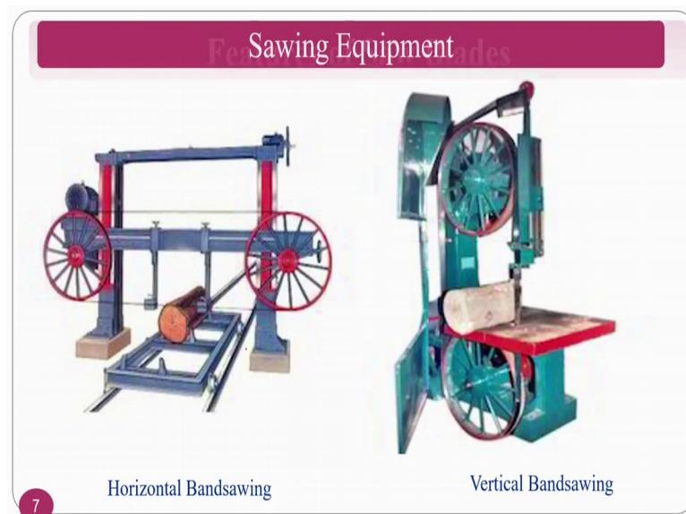
Then equipment if you see there is a horizontal band saw will be there and there will be a vertical band saw. Apart from the hand based hacksaw if at all you are going for the mechanical based or equipment based in that circumstances, you will have two types of band saw where the previous slide you have seen the blade just you mount the blade on either you vertical or horizontal band saw and you can use it.
