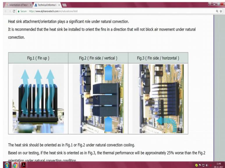
Now, this comes to the other way of a looking at these things. So, we have you know vertical and horizontal; so 1, 2, 3. So, they have given here based on our testing if the heat sink is the thermal performance is 25 percent worse than in the other figure meaning. If you oriented something vertically meaning the fins are like this. So, I have a thing here, I will just show it to you I have a sample here.
