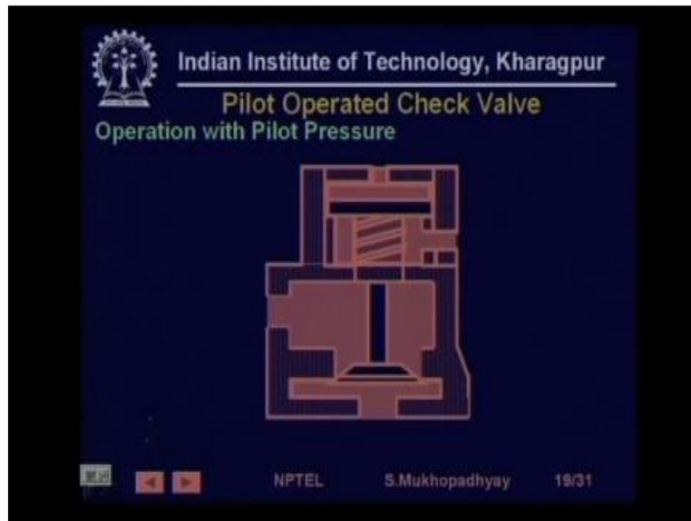
So when we have pilot pressure then this is the pilot port so you have pressure so this spring will be pressed and this will actually come out at the bottom not like exactly aligned maybe somewhere over here so now the fluid now this opening is opened this these openings are open so the fluid will pass and can flow through these they can also fill opens they can also get drained okay so you see so this is a typical pilot operated check valve similarly.
