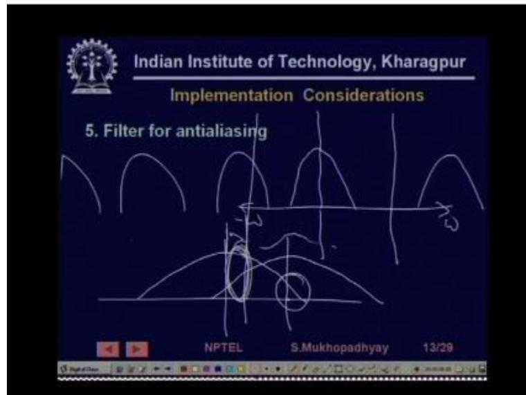
So if you if you take a signal which is which is low pass so its spectrum this is  $\omega$  minus  $\omega$  complex spectrum we are talking about so if a spectrum is like this then and if you are sampling it at this rate then it gets repeated actually the spectrum of the sampled signal is going to be repeated so it will be repeated repeating indefinitely, okay. So now imagine that if you want to if you make this if you make the sampling frequency low.
