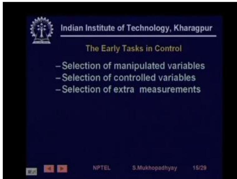
Which variables are to be manipulated selection of controlled variables which variables are to be controlled selection of extra measurements sometimes required or you know choice is required for achieving good control performance like disturbance rejection as we have seen in the case of Cascade loops so how are you going to do the cascade which are the variable you want to sense and feed it as an inner loop feedback you need to understand that.
