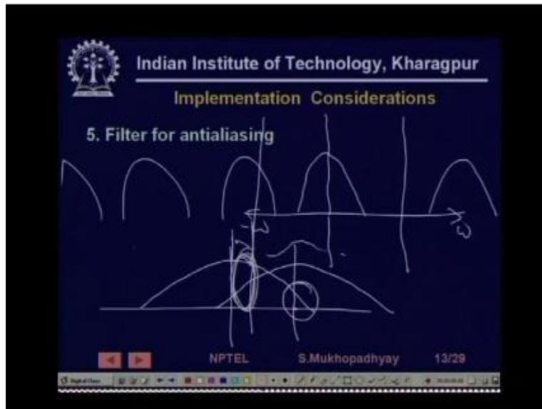
You first cutoff the analog signal such that the high frequency part cannot fold back to the low frequency part so for that purpose you need filters and such filters are called anti-aging filters so you need such filters we must remember that.
