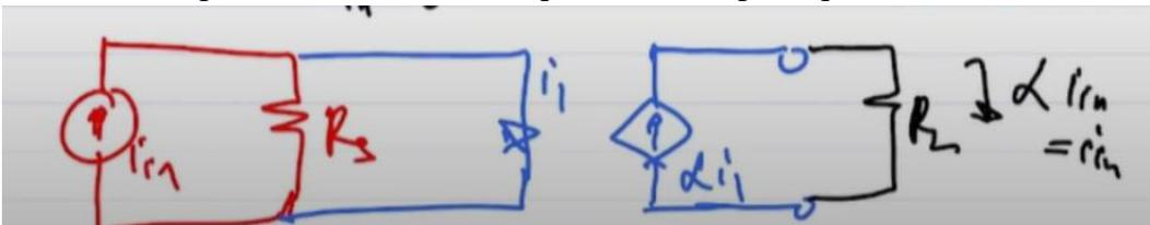
So, the current that flows into  $R_L$  is independent it is not dependent on the effect of loading of the  $R_L$  on the non-ideal current source  $I_{in}$ . So, hence this is a this is the job of a current buffer to translate the current at one port into the other port without causing any loading.
