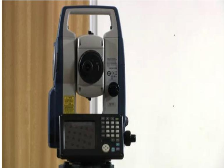
So, in case of total station the measurement of vertical angle like its horizontal angle are automatic. So, if we make it perfectly horizontal then and the telescope or if we make it perfectly to our zenith direction then we will get the zenith angle 0. And when we will make it perfectly horizontal the axis of the telescope then we will get the zenith angles 90 degree. So, these were we get the vertical angles but.
