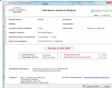
So, what is the right thickness, what do you need to decide on the right thickness of glass? We need what should be the glass size, and how you are going to fix it whether it is 2-side support or a 4-side support, and what is the windload factor that is effecting on the panel. So, there are softwares available which can tell you whether the thickness we have selected is safe or not. So, I recommend you to ask the glass manufacturer for the right thickness of glass.
