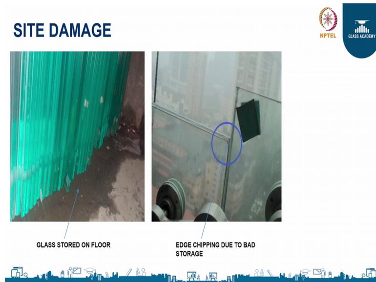
Again you can see glasses were kept floors without any cushion. So, see the floor is wet so, there it might damage the glass again on the see there is a glass to there is edge chip due to bad storage.
