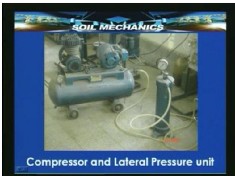
Here we have slightly closer views of the compressor and the lateral pressure unit. Compressor develops the air pressure that is required to drive the water and the pressure into the cell, from here the air pressure comes through this and the pressure is applied to water which goes out through this into the triaxial cell.
