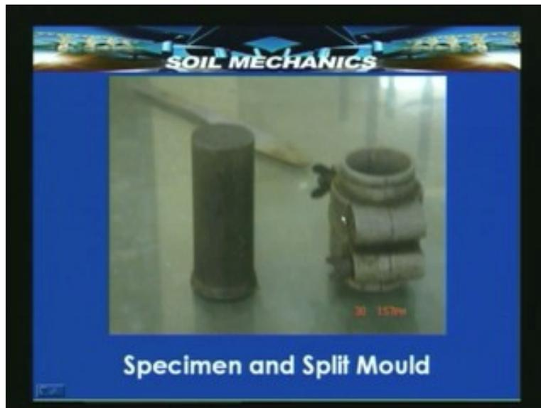
Here is where we have this specimen and this specimen is taken out of the split mould that is if you go back to the earlier slide, when you extract with the help of a plunger the core out of this cylinder then what comes out is collected in a split mould and then because its a split mould, you can open it out and take the sample out and once the sample comes out you can cut it to appropriate sizes and together with this patterns it can be put on the loading machine.
