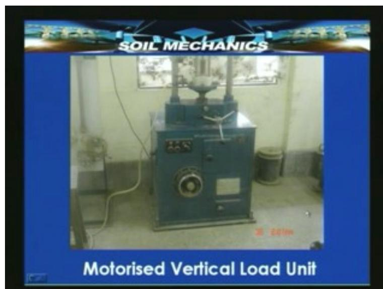
Another photograph, a greater detail of the motorized vertical loading unit. We have here the facility to control the speed of this motor so that the movement in the platen upwards is
