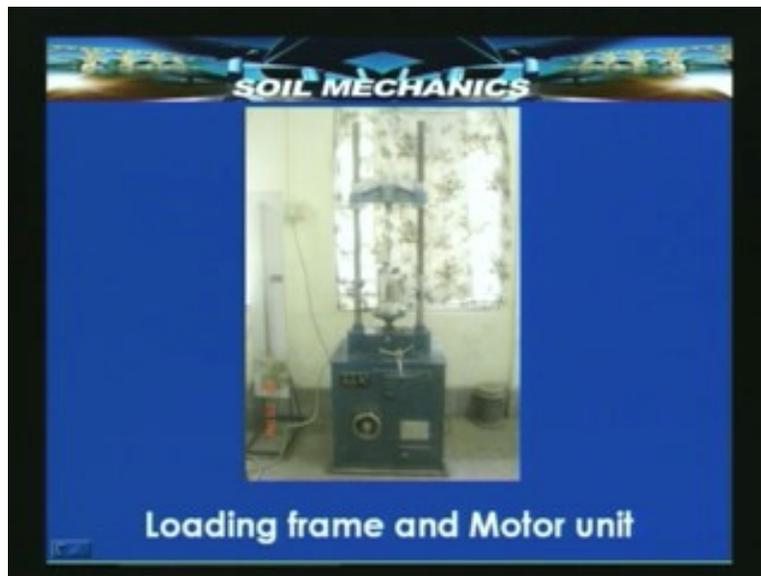
Here is the loading frame, the cell and the motorised unit and the pore pressure unit altogether, one of these views.
