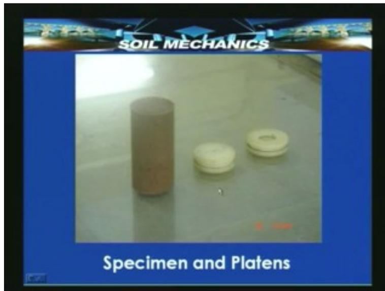
Here we have the closer view of this split mould and the specimen holder in the triaxial apparatus. Now what are the kinds of stresses and strains that develop in the triaxial test when we apply the so called the radial pressure and the axial pressures. So first the self-pressure is applied in the form of a radial pressure and then the pressure is increased in the axial direction until failure take place. So the radial pressure is say  $\sigma_r$  and the axial stress is say  $\sigma_a$ .
