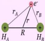
$$\left( -\frac{\hbar^2}{2m_e} \nabla^2 - Q \frac{e^2}{r_A} - Q \frac{e^2}{r_B} + Q \frac{e^2}{R} \right) \psi = E \cdot \psi$$
