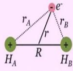
$$\hat{H}(H_2^+) = -\frac{\hbar^2}{2m_A} \nabla_A^2 - \frac{\hbar^2}{2m_B} \nabla_B^2 - \frac{\hbar^2}{2m_e} \nabla_e^2 - Q \frac{e^2}{r_A} - Q \frac{e^2}{r_B} + Q \frac{e^2}{R}$$
