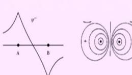
The diagram shows the antibonding molecular orbital wavefunction  $\psi_2$  as a curve that is positive near nucleus A and negative near nucleus B. To the right, the probability density  $|\psi_2|^2$  is shown as two separate circles with a node between them, representing destructive interference of the atomic orbitals.
