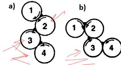
Figure; a) Four roll inclined Z-type
