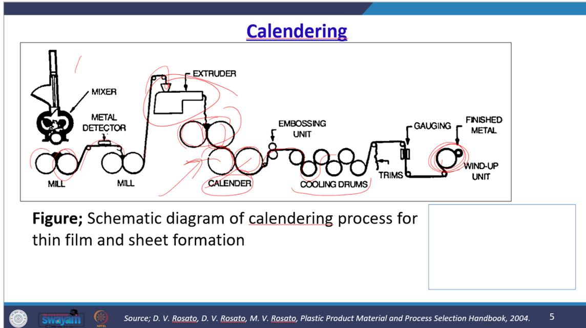
During the calendaring operation, additional features such as embossing, watermarks, and intricate details can be incorporated into the material. Cooling drums play a crucial role in preventing film deformation by maintaining an optimal cooling temperature. Following this, the material undergoes trimming and gauging processes before being wound up on the winding-up unit. This schematic diagram provides a comprehensive overview of the key steps involved in the calendaring process.
