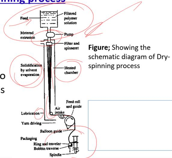
Figure; Showing the schematic diagram of Dry-spinning process
