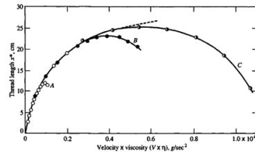
Figure; Showing relation in thread Length vs velocity x viscosity
