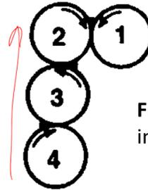
Figure; Four roll inverted L-Type
