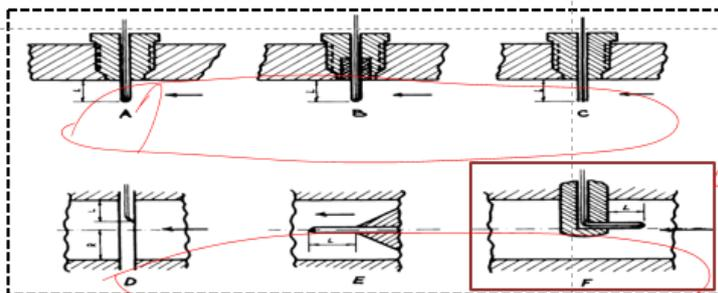
Fig: Placement of thermocouples for temperature profile measurement
