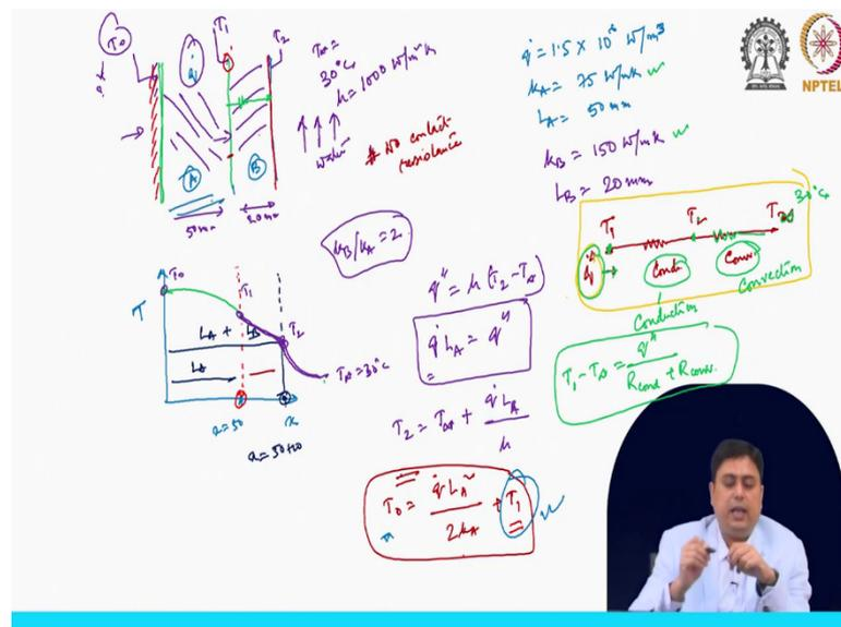
Where the problem was that we had a composite wall of material A material B. The inner surface of material A is the this surface of material A is insulated, material A has a certain thickness, material B has a different thickness the temperature outside of material B is say cooled by a water by water that is having a temperature  $30^\circ\text{C}$ .
