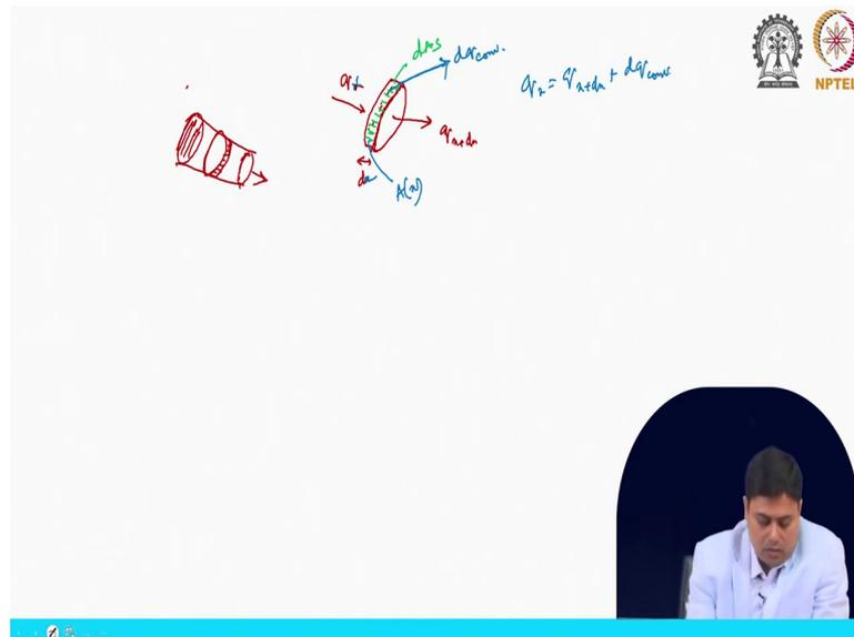
Let us consider a simple scenario where we have a non-uniform case and we consider this differential element where it is attached to the base that mean this is the base surface it is attached to original surface and this is the surface that is exposed to the flowing fluid.
