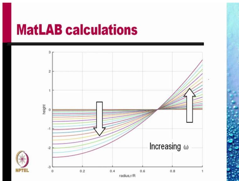
Here I have done/ calculated the free surface for various values of omega. The horizontal line is for zero speed. And as omega increases, at the center the free surface dips and near the wall it climbs up.
