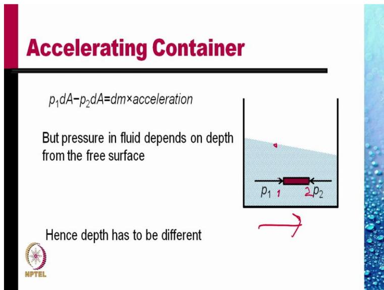
Let us consider a container which is accelerating in the horizontal direction. Consider a horizontal fluid element or cross-sectional area  $dA$ . The net force on this fluid element in the horizontal direction is  $p_1 dA$ , where  $p_1$  is the pressure on the left face *minus*  $p_2 dA$ , where  $p_2$  is the pressure on the right face and this should be equal to the mass of the fluid element times the acceleration.
