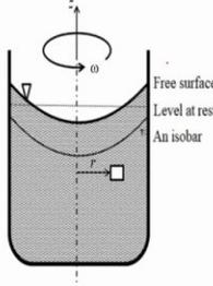
Next, we consider a rotating container. A container of a liquid which is rotating about x-axis at an angular speed  $\omega$ . We see that the free surface of this is curved. If this was the level at rest, then when it is rotating with  $\omega$ , this curved line becomes the free surface. Again, we consider this small element shown as white at the radius  $r$  from the axis.
