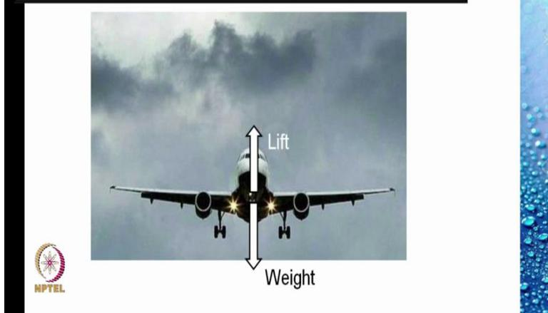
The lift is also responsible to keep an airplane flying in the air. It is the lift generated by the relative motion of the airplane with respect to surrounding air that exerts a vertical force on the wing, normal to the direction of motion of the aircraft. It is this lift which is upwards that balances the weight of the aeroplane.
