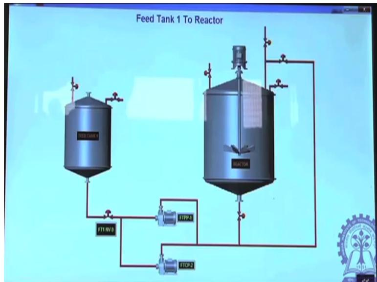
The plant is also equipped with a PLC controller which enables manual controls of individual processes of the plant, further an online monitoring system of various parameters such as temperature pH and the control of processes such as feed transfer to various reactors and the nitrogen supply etc is possible through the software.
