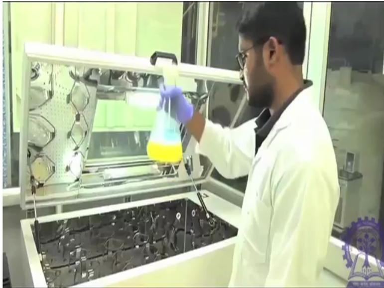
This organism takes up to 10 hours to attain the mid log phase which is ideal for the hydrogen production. In order to facilitate the growth of this organism this media is kept in a incubator shaker up to 10 hours, following the growth which can be visually seen in terms of turbidity of the media, this culture further acts as inoculum for the subsequent bioreactors.
