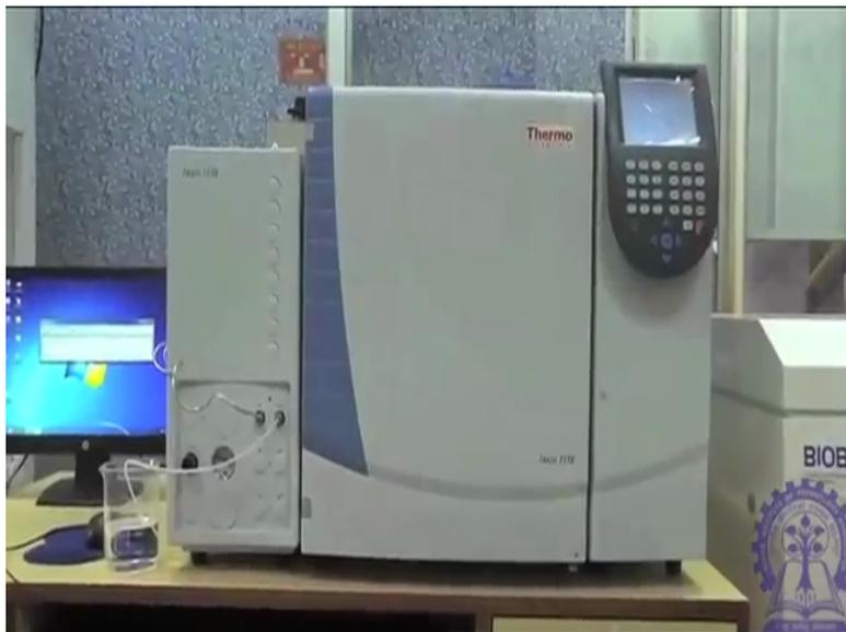
A flow meter installed along the pipeline constantly measures the production rate of the gas inside the reactor. In case of excess gas production the gas can be exhausted through the flame arrested to the atmosphere, gas chromatography is an instrument which is used to analyse the purity of gas. An online gas analysing system is equipped with gc to check the composition of the gas produced in the reactor.
