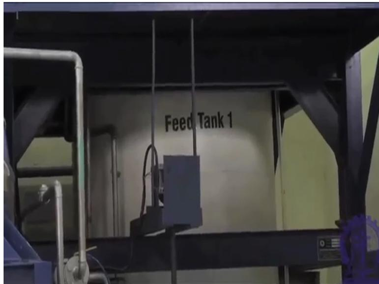
The plant is equipped with various feed tanks each of a capacity of 3 metre cube, it is also equipped with the seed tank of capacity 500 litre, a bioreactor with a working capacity of 10 metre cube, a gas collector with a collection capacity of 2 metre cube. Different accessories such as pumps, pH monitoring and control system, a flow metre, a steam generator, hot water bath, a compressor and a chiller.
