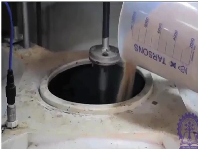
For the media preparation cane molasses is used as the primary substrate, cane molasses is a byproduct of the sugar processing industry. It is a viscous liquid consisting of approximately 40 to 50 per cent of sucrose, so to initiate the operation cane molasses at a concentration of 1 percent volume by volume is added to the feed preparation tank under constant mixing; in addition to the cane molasses groundnut De oiled cake is also added as a nutritional supplement to the media.
