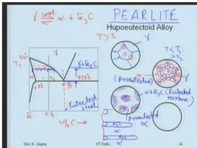
Now looking at the (micro), we have seen the microstructure in one steel but we can talk about this microstructure in other steels as well. If the composition of the steel is to the left of 0.4, I shall have more quantity of the proeutectoid ferrite and less quantity of this austenite which becomes pearlite. It will be still smaller quantity of the islands. So as I go from left to the right, amount of the pearlite is going to increase. By the time I reach at 0.8, it will be 100 percent pearlite.
