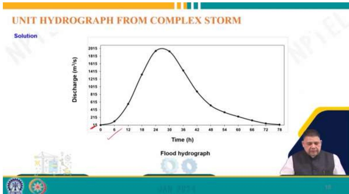
Because it is 15, so it is not starting at 0, but we have started the scale from 15. So, they do not get confused; there is a base flow component of 15 and so on throughout 15, 19, 17, 19, and so on and so forth. So, this is how we can get the unit hydrograph from complex storms.
