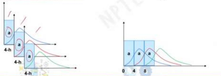
So, coming to the method of superposition, we have a 4-hour unit hydrograph, and we wish to develop a 12-hour Intergraph, that means  $n$  is equal to 3, D-hour to ND-hour, we said  $n$  equal to 3. So, we need to in that case, we need to superimpose 3 4-hour unit hydrographs each lagged by 4 hours from the previous one.
