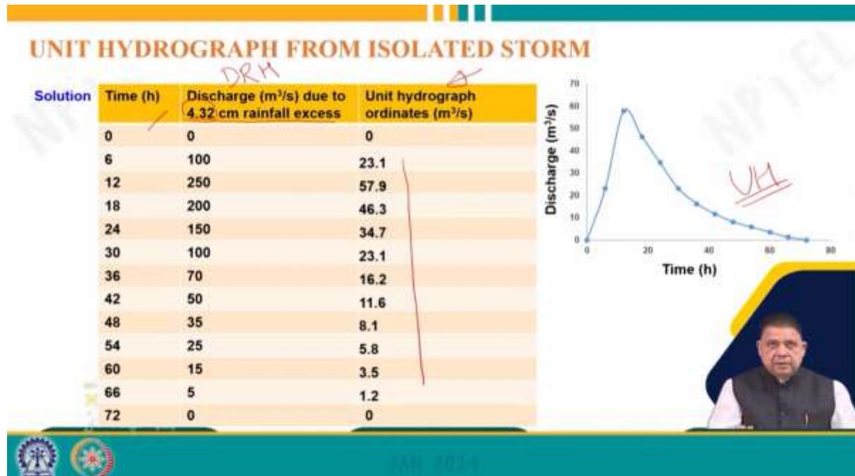
Now, we have time and we have discharge due to the 4.3 centimetres of direct runoff rainfall excess, which is nothing but the DRH. These ordinates are nothing but the DRH ordinates given to us. So, for getting the unit hydrograph ordinates, we have to divide each ordinate by this effective rainfall depth, which is 4.32. That is what it is.
